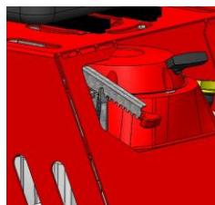
Fig. 19: Rotating speed regulation
